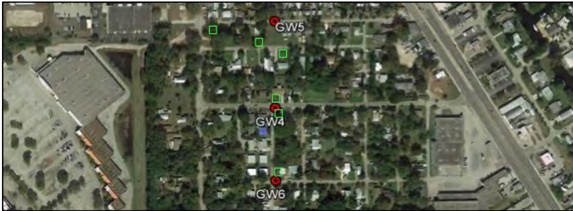
Figure 10. Groundwater monitoring wells (GW4-GW6) located near the “central drainage feature” in North Fort Myers, FL; the approximate location of some septic tank drainfields are indicated by the green squares. Not all drainfields in this area are represented in this map due to a lack of information.
